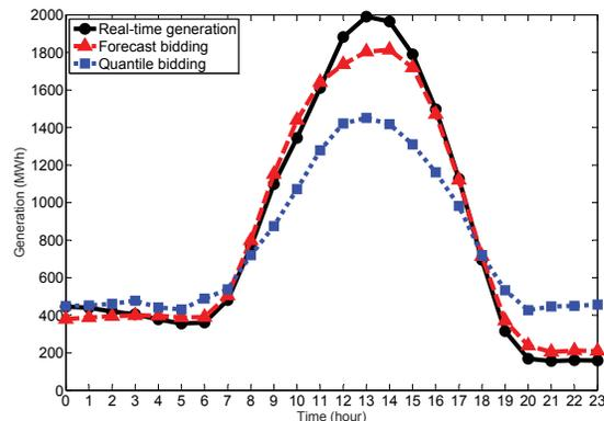
Fig. 4. Data on 1 May 2016 represent coalition-based quantile and forecast biddings as well as real-time measured power in the grand coalition [17].
