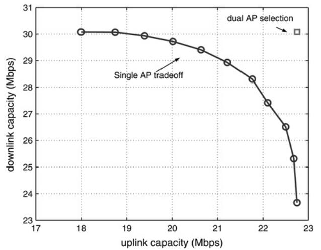
Fig. 11 Ergodic capacity region of uplink and downlink for different  $\theta$  (19-cell scenario)
