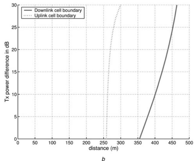
Fig. 6 Impact of relaying cost on the cell boundaries
