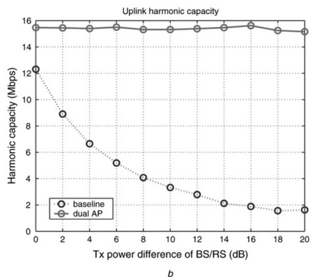
Fig. 9 Uplink capacities in a 19-cell scenario
