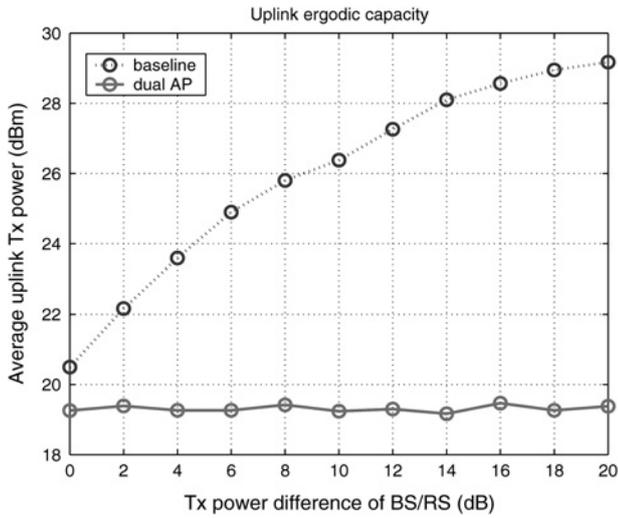
Fig. 10 Uplink Tx power saving in a 19-cell scenario
