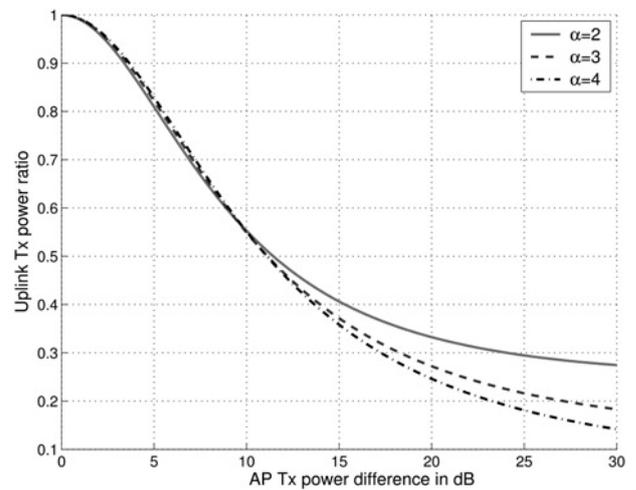
Fig. 3 Reduced Tx power using dual APs
