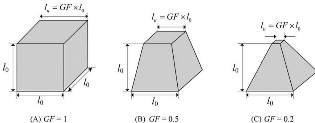
**FIGURE 5** The target geometries for a cube and two trapezoidal hexahedrons are described. The baselines and heights are retained as  $l_0$ , while  $l_u$  is determined by the GF
