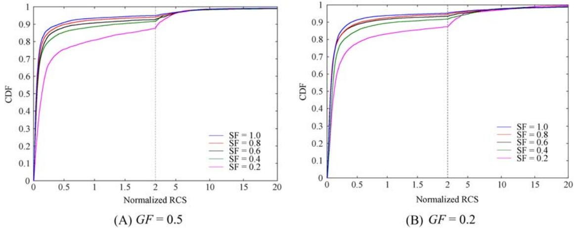
**FIGURE 6** CDFs with  $GF = 0.5$  and  $GF = 0.2$  are plotted for selected SFs, respectively. Note that two different scales are used to emphasize the CDFs with low RCSs. [Color figure can be viewed at wileyonlinelibrary.com]
