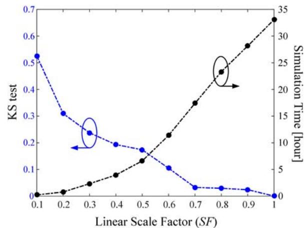
FIGURE 3 K-S tests and simulation times as a function of the SF. The K-S tests agree when  $SF > 0.7$ , and the simulation time of  $SF = 0.7$  is reduced to 52.6% compared to  $SF = 1$ . [Color figure can be viewed at wileyonlinelibrary.com]
