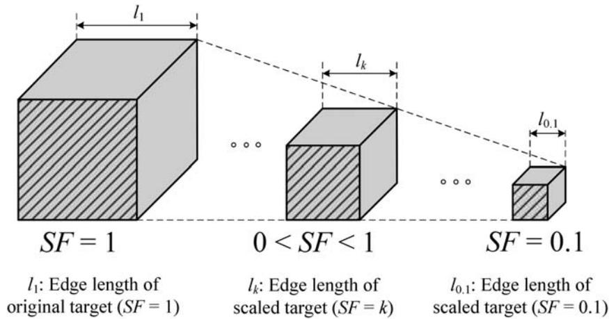
FIGURE 1 Original and downscaled target cubes. SF varies from 1 to 0.1 by a step of  $-0.1$
