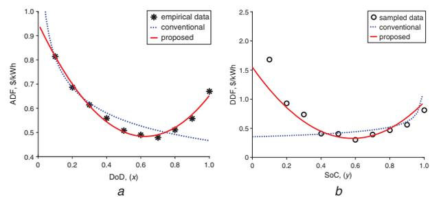
**Fig. 2** ADF and DDF of empirical data, conventional method and proposed method for battery A
