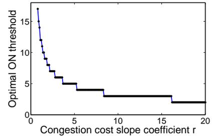
**Figure 8: Optimal ON threshold over  $r$  for  $\rho = 20\%$  and  $E_{ch} = 1.16 \times 10^{-4}$  kWh. When  $r$  increases, the emphasis on congestion cost increases as well and the hysteresis decreases.**
