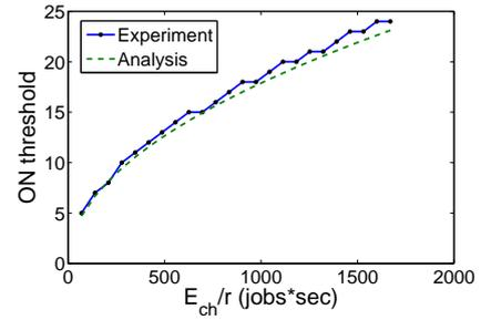
**Figure 7: Optimal ON threshold over  $E_{ch}/r$  for  $\rho = 20\%$ . When  $E_{ch}$  increases  $ON \rightarrow OFF$  and  $OFF \rightarrow ON$  switchings become more energy consuming. The hysteresis increases to avoid frequent  $ON \rightarrow OFF$  and  $OFF \rightarrow ON$  transitions.**
