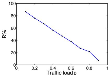
**Figure 10: Fraction of energy saved over traffic load  $\rho$  for  $r = 3$  Joules/sec and  $E_{ch} = 1.16 \times 10^{-4}$  kWh.** The percentage of energy saved is reduced with traffic load, since increased number of jobs reduces the server sleeping time.
