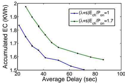
**Figure 9: Pareto-optimal curve for energy consumption and average delay tradeoff:**  $E_{ch} = 1.16 \times 10^{-4}$  kWh and  $E_{ch} = 1.98 \times 10^{-4}$  kWh ( $\rho = 20\%$ ). Each curve is obtained by varying the congestion cost coefficient  $r$ . When  $E_{ch}$  increases, the system's performance becomes poorer.
