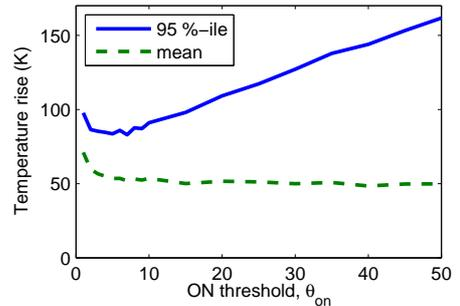
**Figure 11: Temperature rise over ambient, as a function of ON threshold, for  $\lambda = 10$ ,  $s = 50$ ,  $C_{th} = 1$ ,  $b = 1$ .** After some point, the 95 percentile of the server temperature rise (compared to ambient temperature) increases with  $\theta_{ON}$ . Higher energy savings increase the probability of damagingly high temperatures.
