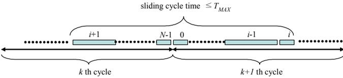
Fig. 2 Sliding cycle time constraint
