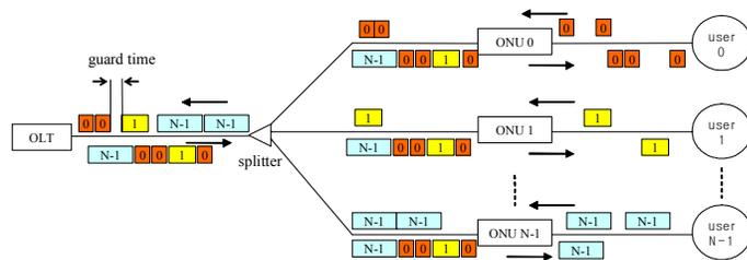
Fig. 1 Point-to-multi-point topology of EPON
