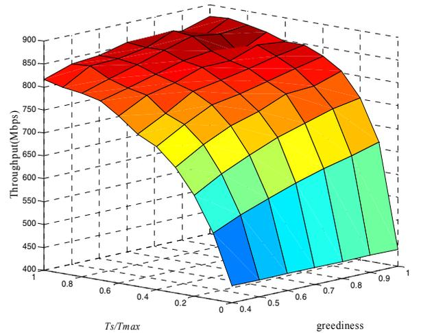
Fig. 6. Throughput for various  $\gamma = T_S / T_{MAX}$  and greediness  $\alpha_i$ . Test ONU transmits 950 Mbps while 15 ONUs are idle. Note that  $\gamma = 0$  stands for IPACT.
