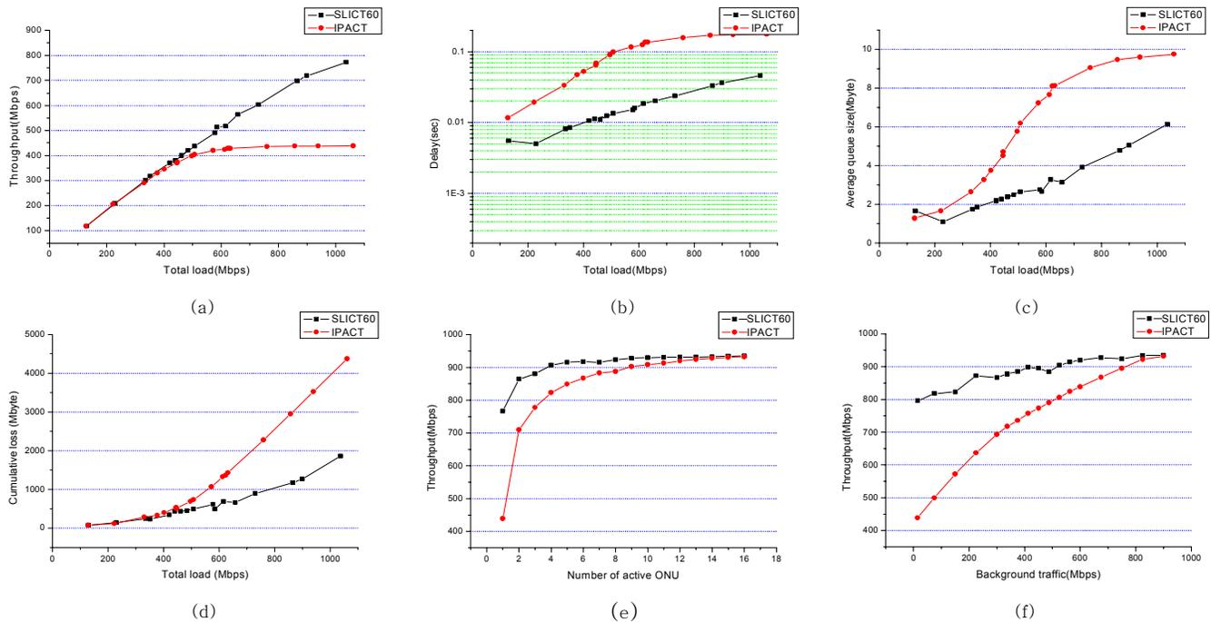
Fig. 7. Test under  $C_i$  is 60 usec and  $\alpha_i=0.9$ . (a)-(d) Performance of SLICT and IPACT when one ONU sends from 50 to 950 Mbps while 15 ONUs are idle: (a) Throughput (b) Delay (c) Average queue size (d) Loss (e) Aggregated throughput of  $M$  ONUs equally sharing the uplink (f) Aggregated throughput when 15 ONUS send background traffic from 0 to 950 Mbps while one ONU sends 1G – background traffic, so the aggregated load is 1 Gbps.
