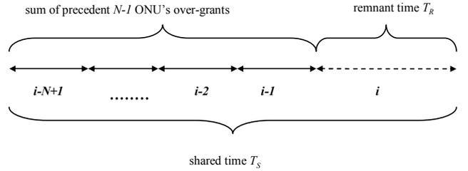
Fig. 3. Calculation of the remnant time  $T_{R,i}$  from the shared time  $T_S$  and over-grants  $O_j$   $\{j = i-N+1, \dots, i-1\}$
