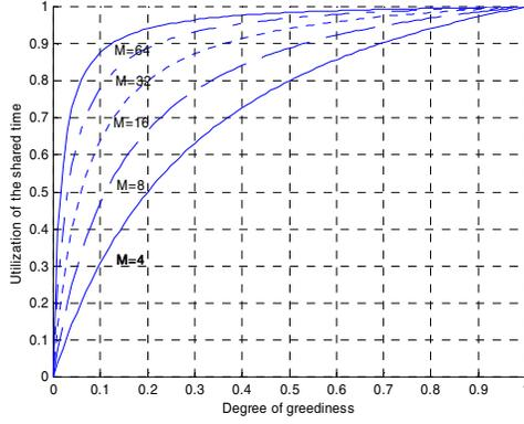
Fig. 4. Utilization of the shared time in steady state when  $M$  ONUs are over-loaded
