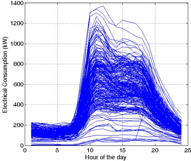
Fig. 2. Typical load curves of the industrial building.
