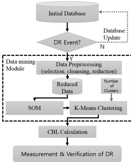
Fig. 1. Framework of the baseline load computation.
